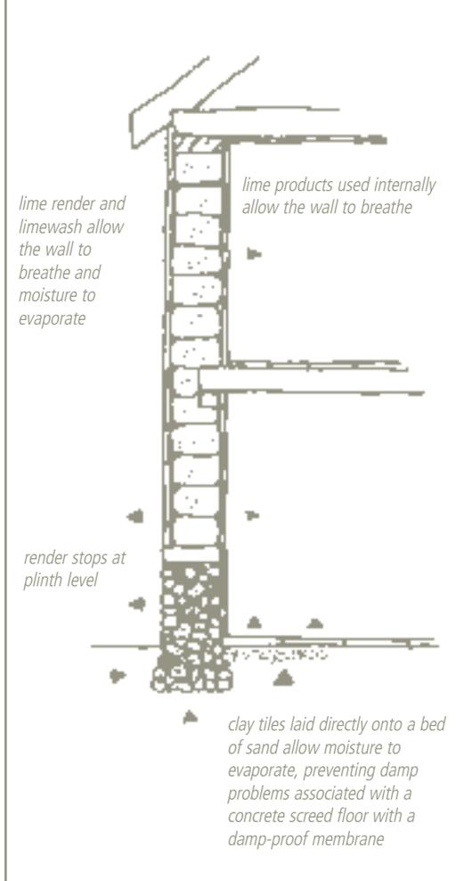
By changing the materials of the building by replacing a lime render with a cement render or a timber floor with a concrete floor, for example, the special breathable qualities of an historic building can be damaged, leading to problems of damp and decay.
