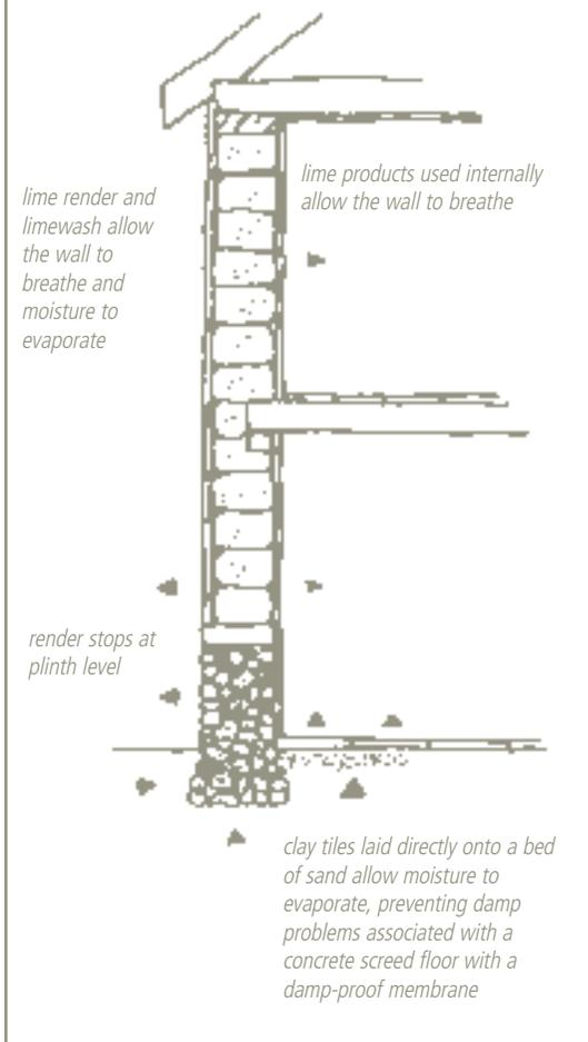
By changing the materials of the building by replacing a lime render with a cement render or a timber floor with a concrete floor, for example, the special breathable qualities of an historic building can be damaged, leading to problems of damp and decay.
