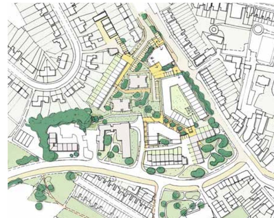
Fig.56 Partial demolition combined with infill homes
