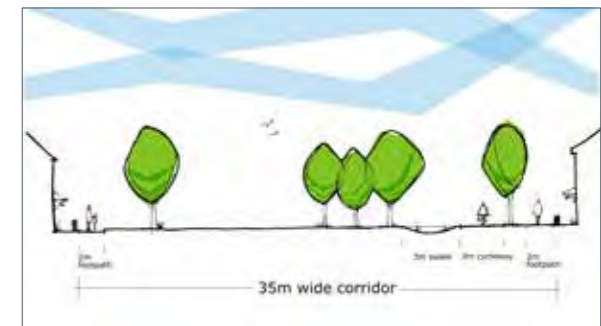
Section through Central Green Space
