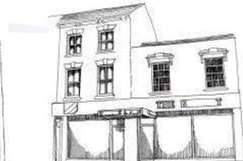
A shopfront unsympathetic to the building
