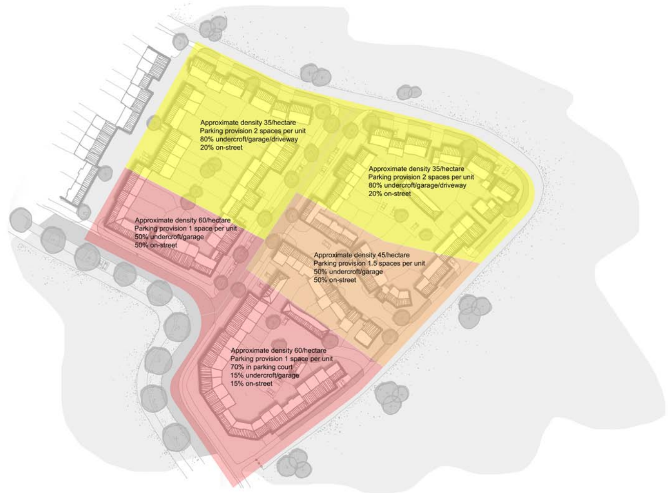
Example block demonstrating how numbers and parking provision can be accommodated within a variety of street typologies and densities.
