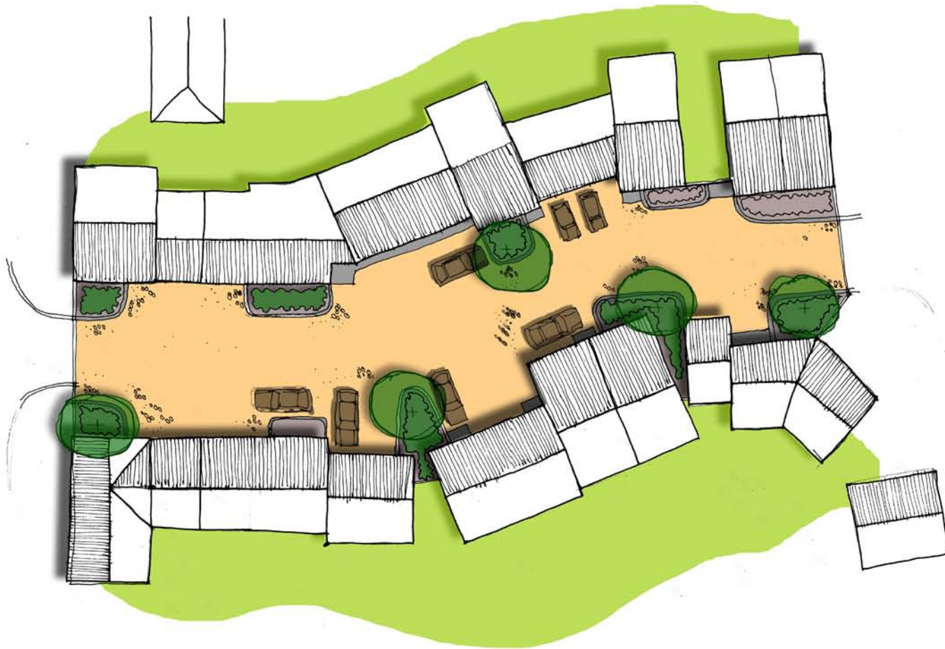
Concept sketch showing the arrangement of a typical Rural Mews. The scale is similar to a mews but the spaces include more areas of planting.
