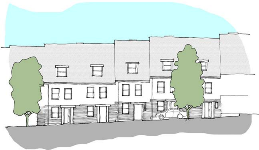
Elevation showing how the built form can respond to level change in higher density areas, where the gradient is approximately 1:15.
