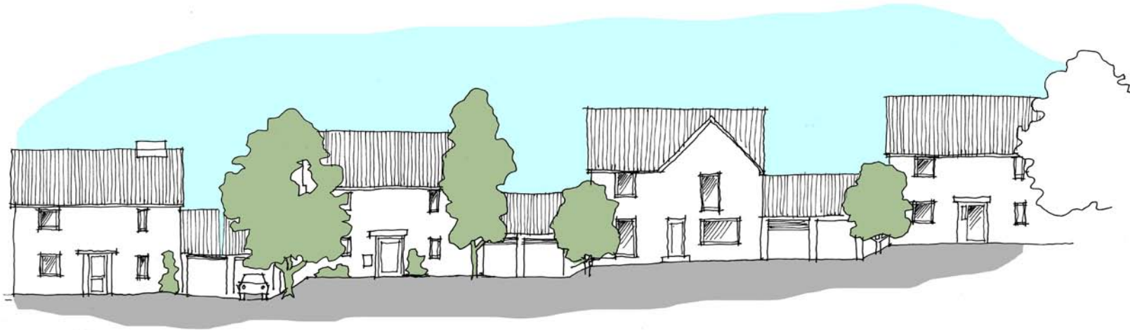
Elevation showing how built frontage can accommodate level change in lower density areas, in areas of highest gradient (approximately 1:15 slope)
