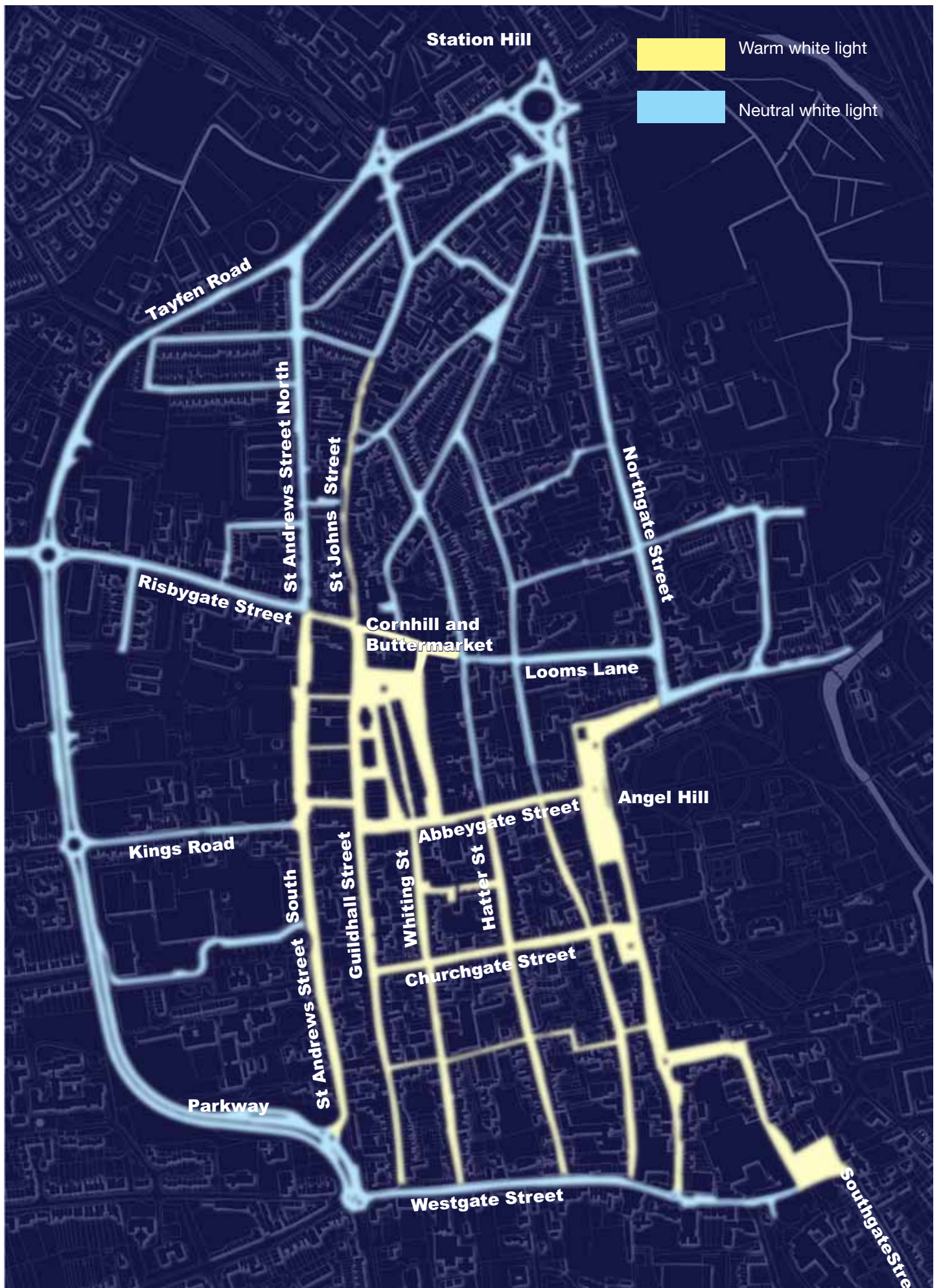
Figure 19 : Streets - colour temperature diagram
