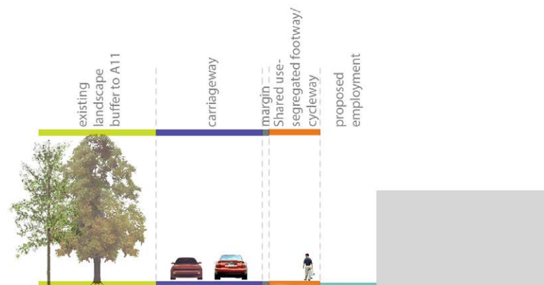
FIGURE 26 INDICATIVE ACCESS ROAD SECTION
