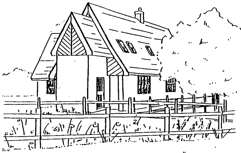
Recently constructed housing in St. John's Street, Beck Row which is a modern interpretation of a traditional rural cottage; steeply pitched roof, narrow gable, low eaves, additive building form, chimney. However, the development could have benefited from more landscaping and darker stained timber boarding.
